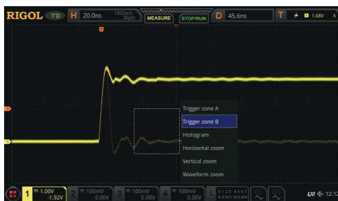
Draw a rectangle on the transient exception signal and select Trigger zone A.
